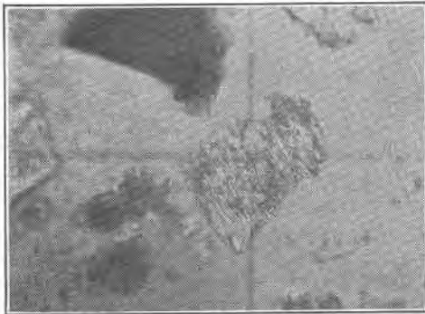
Fig. 4. Andalusite, cone 13. The grain in the center of the preceding photograph magnified to 315 times, showing the detail of the parallel fibers of mullite extending across the grain.
