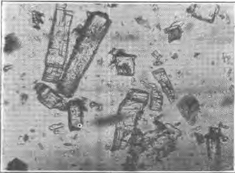
Fig. 8. Cyanite, cone 10. Note the clear undecomposed grains and cleavage cracks. The black grains are mica as in Fig. 1. Magnification 90.
