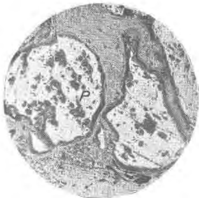
Figure 1. Rounded fragments of pyrite (P) partially altered to limonite, 9th level, Old Dominion mine, Globe, Arizona. Mag. 52X
