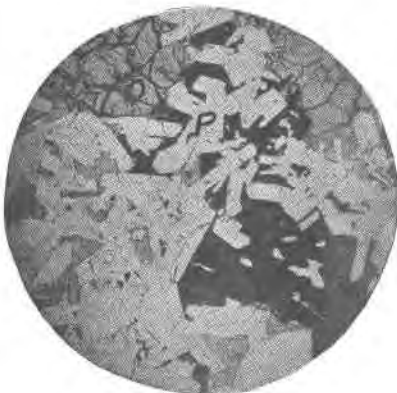
Figure 12. Micrograph of a thin section of a sulphide diabase. Note fresh olivine (O), augite (A) and plagioclase (P). Euhedral feldspar crystals are embedded in sulphides (black). Exploration pit, Cook County, Minnesota. Mag. 16X.
