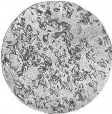
Figure 7. Rounded fragments of pyrrhotite (Pr) in galena. A primary ore showing replacement. Sullivan mine, Kimberley, B. C. Mag. 33X.
