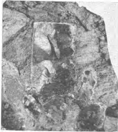
FIG. 1. Crystal of uranothorite (X 3) showing thin white line of alteration products next to matrix.
