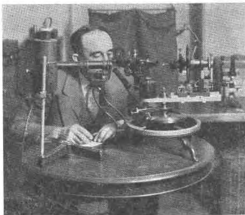
FIG. 1. Goniometer mounted on rotating table.
