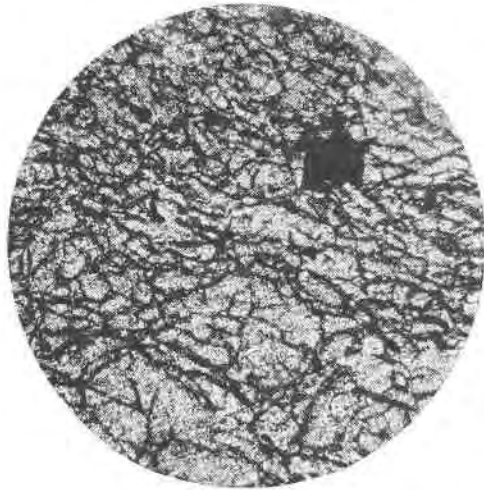
FIG. 1. Highly magnified photograph by transmitted light of a thin section of Sabine township euxenite, showing regular fracturing and freedom from inclusions. The black spot represents a hole in the section. The photograph does not give a true picture of the section. Actually the fractures are very narrow and sharp with little or no alteration along the edges.
