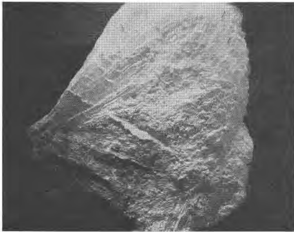
FIG. 2. Probertite in massive borax. Magnified 1\frac{1}{2} diameters.
