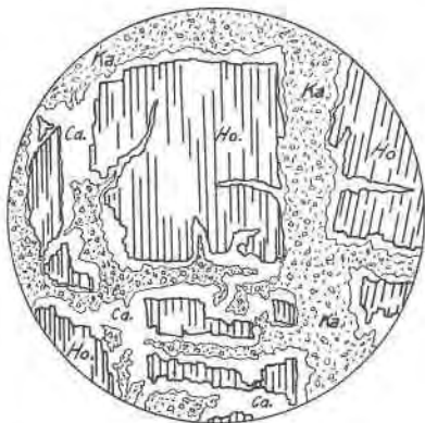
FIG. 6. Drawing of thin section \times 25 . Hornblende (Ho) subjected to attack and filling by calcite (Ca) and later removal of portions of the calcite with the formation of kaolinite.
