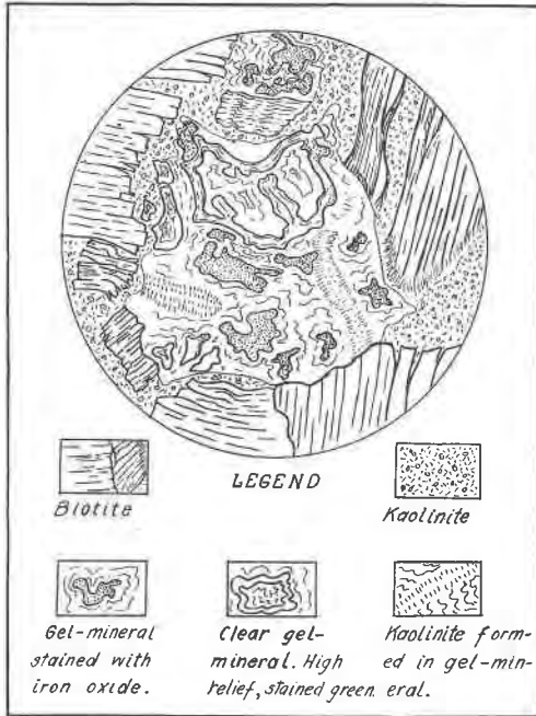
FIG. 10. Drawing of thin section \times 25 . Progressive alteration in micaceous portion of the rock to form kaolinite. An isotropic brown gel-mineral is first produced which grades into a green gel-mineral phase. The latter grades in turn into a pale green gel-mineral which grades into kaolinite. The progressive loss of color and structure in the sequence of gel-minerals suggests reduction and removal of iron.
