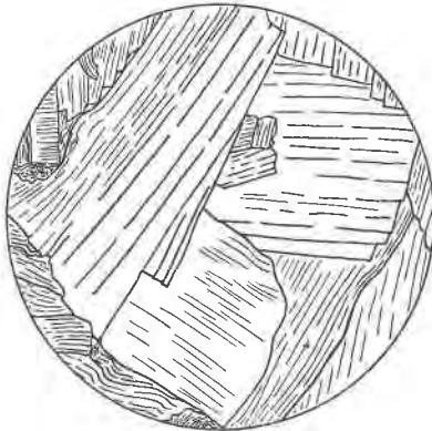
FIG. 8. Drawing of thin section \times 25 . A mass of green vermiculite which, judging from color variations in adjacent areas, is an alteration of biotite.
