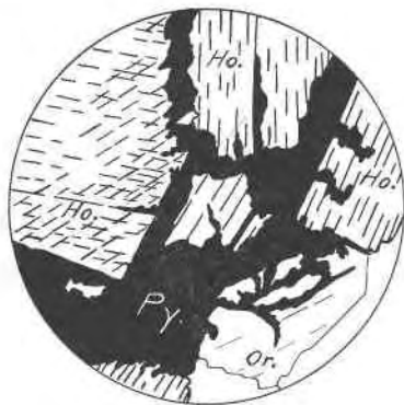
FIG. 4. Drawing of thin section \times 25 . Hornblende (Ho), Orthoclase (Or), and Pyrite (Py) are the minerals present. A portion of the granodiorite containing a concentration of pyrite probably "magmatic" but later than the silicate minerals.
