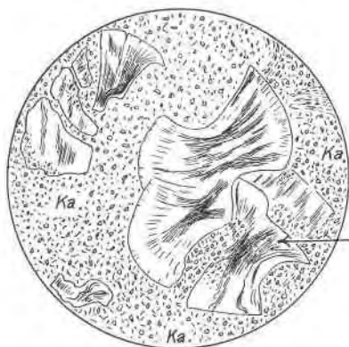
FIG. 9. Drawing of thin section \times 25 . Remnant structures originally biotite but now kaolinite within a ground mass of kaolinite. The sheaf-like structure is apparently due to the marginal expansion of the mica flakes, during the replacement. The streaks are dark colored residual stains. (Indicated by the arrow.)
