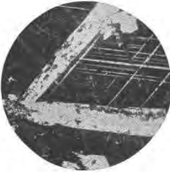
FIG. 6. Coarsest plates of ilmenite observed in magnetite. South of Snowbank Lake, Minnesota. Mag. X 73 (Etched).
