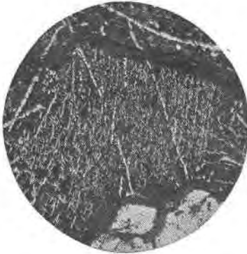
FIG. 2. Fine dash type of ilmenite intergrowths in magnetite. Tucker Lake, Minnesota. Mag. X 73.
