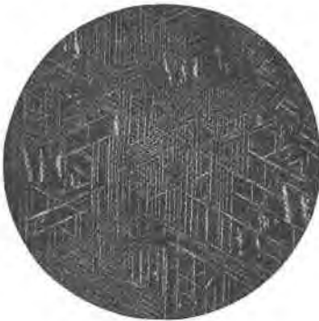
FIG. 4. Closely crowded ilmenite plates along the parting of magnetite. Essentially the Widmanstätten structure. Tucker Lake, Minnesota. Mag. X 80.
