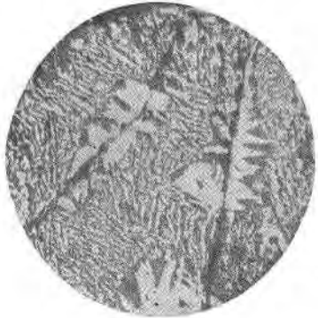
FIG. 9. Graphic intergrowth of ilmenite (white) and hornblende. Anorthositic gabbro, (unetched). Duluth, Minnesota. Mag. X 112.
