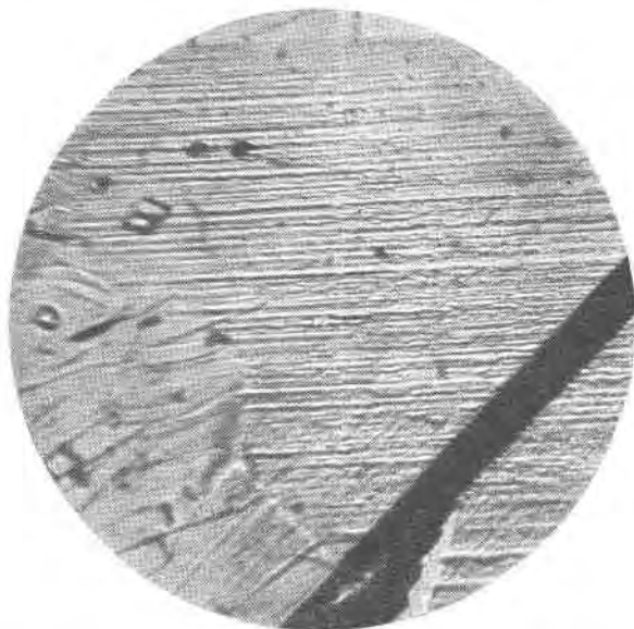
FIG. 4. Parallel striations extending across a natural cleavage face of galena at an angle of approximately 45^\circ to the cubic cleavage. Magnification 225\times . The distance between the lines shown is approximately 0.004 mm.
