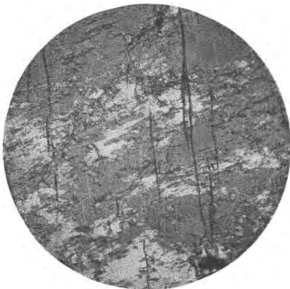
FIG. 2. Sobralite and iron rhodonite, homoaxially intergrown with each other. White=sobralite, grey=iron rhodonite. In the latter twinning lamellae parallel to (010). The partly clouded appearance of the sobralite is due to the presence of small, newly formed inclusions, probably of grünerite. The same mineral is also found as inclusions in the iron rhodonite, arranged along lines parallel to (001). Somewhat larger prisms of grünerite are seen at more points. Magn. 48 \times , crossed nicols.
