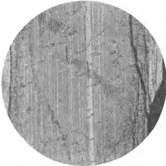
FIG. 6. The same rhodonite as in FIG. 5. Section about perpendicular to \alpha . The white lines represent twinning lamellae parallel to (010). The rhodonite holds the same diopside-perthite inclusions as in FIG. 4, and similar perthite-rich lines as in the latter. Magn. 48 \times , crossed nicols.
