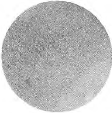
FIG. 7. Pyrargyrite etched by heat and light. Note the concentration of the elongated dashes (etch marks) along the scratches. This pattern is finer than that of stephanite. 4 mm lens, mag. 178 \times .
