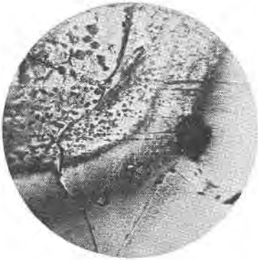
FIG. 9. Andorite etched by the rays from the carbon arc light. The central portion is deeply pitted and fractured, while around this there is a band of red to iridescent colored etching. 4 mm. lens: Mag. 178 \times .
