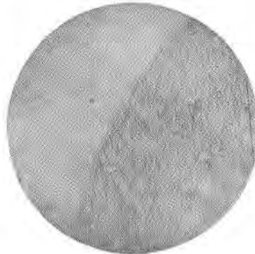
FIG. 6. Stephanite etched by both light and heat. The pattern resembles that of pyrargyrite, proustite, and pearceite, but it usually is coarser. 4 mm. lens. Mag. 178X.
