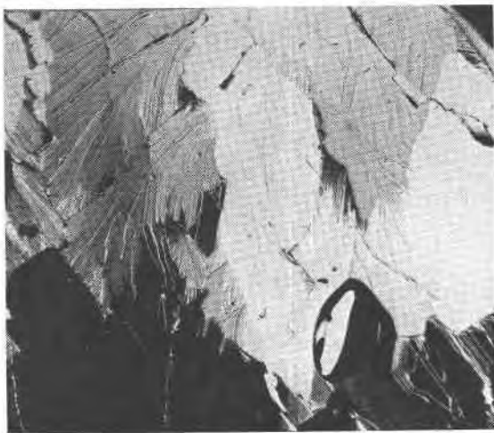
FIG. 3. Cleavage surface of Joplin galena, \times 65 , specimen slightly tipped to display lineages. The two rounded black areas about half an inch across, in the right and left lower centers, are negative crystal cavities. The blocks of various shades and irregular shapes are lineages. The occurrence of negative crystals at lineage boundaries is obvious.
