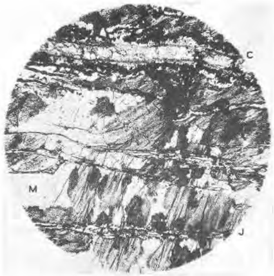
FIG. 10. Melilite (M) altered partly to juanite (J) and cut by a vein bordered by cebollite (C). The centre of the veinlet is mainly filled with fine-grained carbonate. Ordinary light \times 20 .
