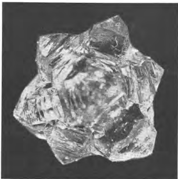
FIG. 1. Photograph of diamond multiple twin viewed from the direction of a trigonal axis. Magnification about 9.
