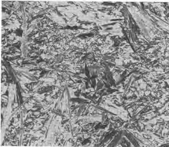
FIG. 2. Photomicrograph of nephrite illustrating the occurrence in long, bladed, radiating fibers. Crossed nicols. \times 27 .
