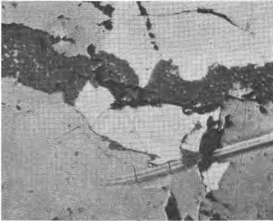
FIG. 3. Veinlet of younger sphalerite (dark gray) with inclusions of chalcopyrite (white) crossing chalcopyrite (white) and pyrrhotite (light gray). Nicols not crossed. Magnification 400 diameters.
