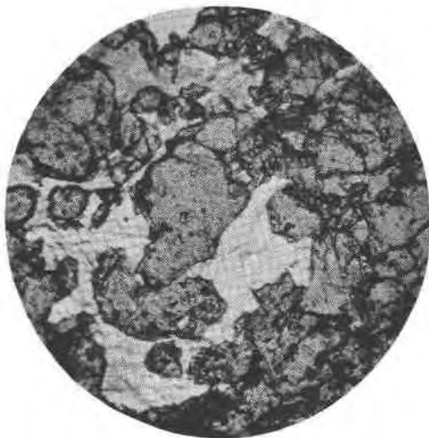
FIG. 3. Section of a garnet-rich veinlet showing later quartz and calcite. Cornucopia, Oregon. 35 \times .
