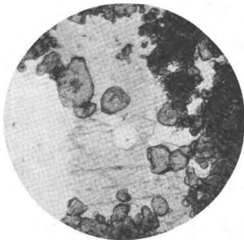
FIG. 4. Another portion of the garnet phase showing a basal section of quartz surrounded by calcite. Snoqualmie Pass, Washington. 35 \times .
