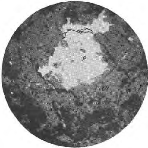
FIG. 4. Photomicrograph of the Beardsley aerolite. Ol. Olivine; P. Nickel-iron; Pyr. Pyrrhotite. This photomicrograph illustrates the variation in smoothness of the olivine-metallic contacts. 60 \times .
