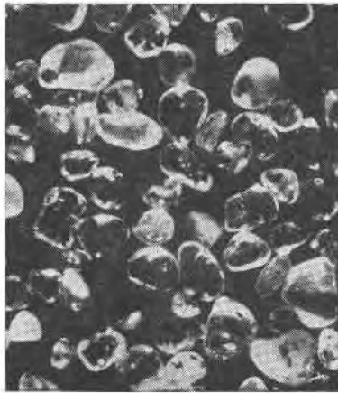
FIG. 4. Transparent sand grains photographed on a red celluloid background. The arc light strikes the grains at a low angle. Reflection of the light from the polished surfaces of the grains illuminated all sides of the grains. A green filter may be used to soften the high lights. Mag. 10\times .
