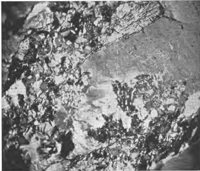
FIG. 2. The large gray grain with the ragged border extending diagonally upward to the right from the center of the view is potash feldspar. It is surrounded by a fine-grained intergrowth of quartz, feldspar, chlorite and epidote, fringed with myrmekite. The appearance of corrosion of the potash feldspar is too obvious to need comment. The light-colored splotchy border of the potash feldspar appears to have been produced by alteration by the corroding solutions. Crossed nicols, \times 30 .
