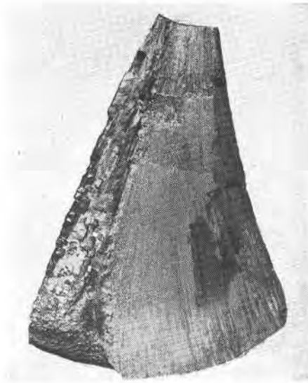
FIG. 1. Specimen of pyrite showing the gradation from cubic crystals into a distinctly fibrous structure. From the Eadie Mine, near Hanover, Illinois. About 2/3 natural size. (Photograph by O. R. Grawe.)
