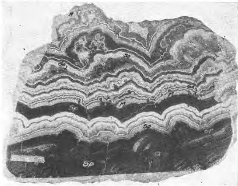
FIG. 3. Colloform bands of zinc sulphide, the bands colored probably by adsorbed iron compounds. Moresnet, Belgium.
