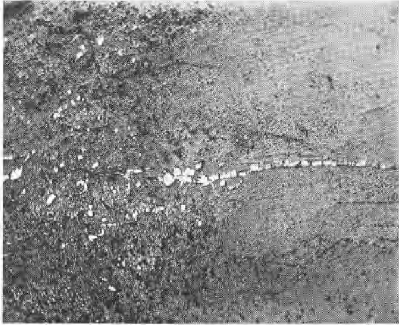
FIG. 3. A veinlet and scattered grains of uraninite. The photomicrograph represents the appearance of a veinlet responsible for one of the streaks in the radiogram. Most of the spots and streaks in the radiogram are due to uraninite of this type. It is not unusual for a veinlet to produce a streak on the radiogram twenty times as broad as the original veinlet. It should be pointed out therefore that the radiogram Fig. 2 gives an exaggerated idea of the actual radioactive area. (Photomicrograph \times 150 .)
