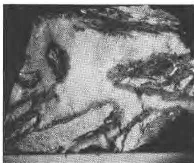
FIG. 12. Same as Fig. 11 but showing inclusions in white vein quartz crossed by piedmontite and, in fact, more completely replaced. \times 0.7 .
