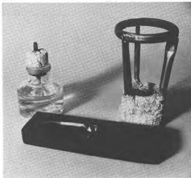
FIG. 1. Charcoal block with platinum spoon, alcohol lamp, and tripod which rests on shoulder of lamp.
