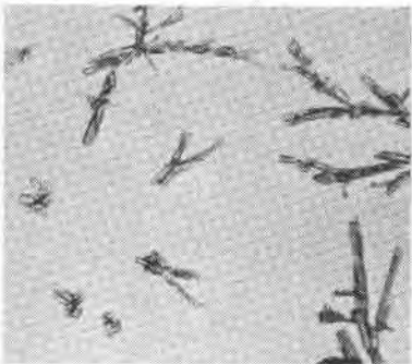
FIG. 5. Boric acid. The plates show low birefringence while the branching forms have higher birefringence. \times 40 .
