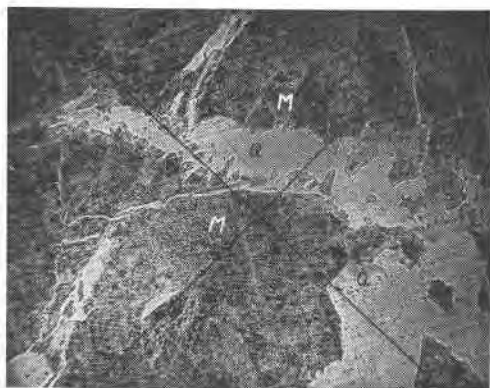
FIG. 3. Quartz (Q) veinlet replacing microcline (M). Note the smaller areas of quartz at the upper center and lower left and the small remnants of feldspar along the margins of the veinlet. Mag. 45 diameters.
