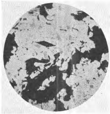
FIG. 3. Photomicrograph of a polished section of the Grace Vein, Darwin Mine, showing idioblastic crystals and veinlets of riebeckite (black) in native gold (light-grey) with inclusions of chalcopyrite (grey). One nicol, \times 560 .
