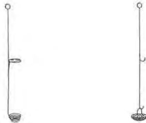
FIG. 2. Double weighing pan for single fragments.
