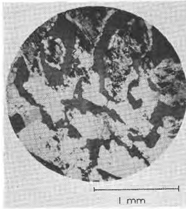
FIG. 2. Photomicrograph of albite graphic granite showing microcline being replaced by albite. Note corrosion of quartz by albite. Albite is white; quartz, medium gray; and microcline, dark gray. Redstone, N. H.
