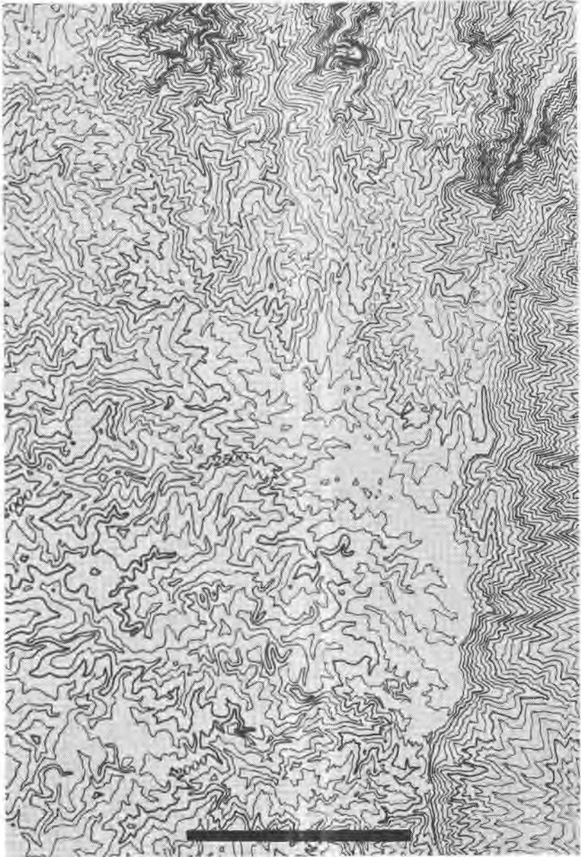
FIG. 3. Contour pattern of the summit of the Koolau Range at the northern end of the area of clay occurrence on Oahu, showing comparatively smooth, little-dissected, probable remnant of constructional surface. To the east is the steep, nearly continuous cliff formed by the heads of windward valleys. The heavy line is one mile long. Contour interval 100 feet. Photograph from the blue-and-brown U.S.G.S. sheet.
