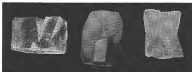
FIG. 3. (01\bar{1}2) twins in calcite; left: "knife blade" twin similar to those illustrated in Figs. 1 and 2. Center: twin-gliding lamellae on a crystal of calcite from Egremont, England. The crystal is bounded by cleavage rhombohedrons and prism faces. Compare with the projection Fig. 4. Right: growth twin from Guanajuato, Mexico.
