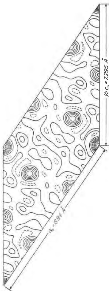
FIG. 3. Fourier projection along the symmetry axis ( b -axis) of the structure of sylvanite. The contour map within the parallelogram represents the projection of one half of the unit cell. The peaks at the corners of the parallelogram represent gold atoms. The peaks midway between the corners along the vertical boundaries represent silver atoms. The peaks along the inclined boundaries and within the parallelogram represent tellurium atoms. Dotted lines are depression contours.
