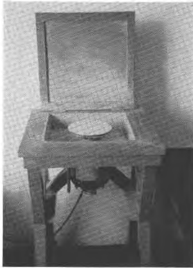
FIG. 11. Paper lap polishing equipment.
