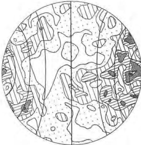
FIG. 12. Wayland's diagram of 155 quartz axes from the St. Peter sandstone. Small circles drawn in for comparison with the theoretical diagram of Fig. 11.
