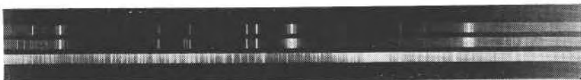
FIG. 10. Spectrograms of natural Colombian emerald (upper strip), synthetic emerald (central strip) and "Armco" iron (lower strip).
