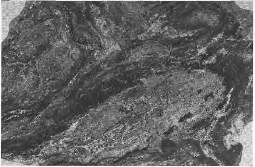
FIG. 2. Dark, beryllium-bearing ribbon rock tactite from Discovery Gulch, Iron Mountain, New Mexico. Black areas are fine-grained silicates stained with manganese oxide; gray areas are magnetite; grayish, irregular pod-like areas are helvite; and the white patches and thin veinlets are fluorite. (Natural size.)
