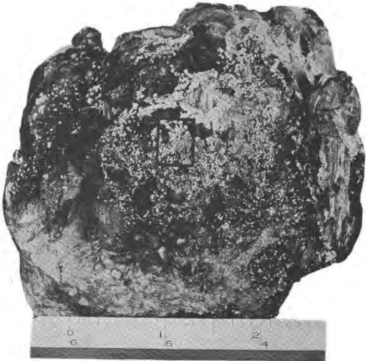
FIG. 2. Manganiferous limonite from Kelly Bank mine, Vesuvius, Virginia, showing specks of weinschenkite on surface of ore. Scale in inches.
