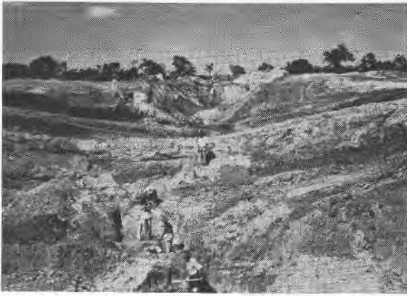
FIG. 2. Looking south along the strike of the vein system at the Guachi mine, near Sete Lagôas, Minas Gerais. Mining of nearly vertical vein by hand methods in foreground. Red overburden has been stripped off and mining will advance to center of picture. Old workings are in background pit on same vein zone although individual veins pinch out along the strike.
