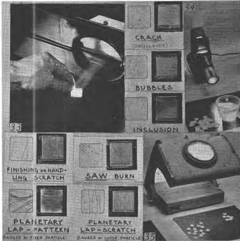
FIGS. 33-35. Among the most important stages of inspection in processing are those of the blanks prior to lapping and prior to final finishing. Prior to lapping, blanks are inspected for internal imperfections (cracks, bubbles, inclusions) by immersing the blanks in oil and scanning them in an intense spot-light (Figs. 33-34). Prior to etching to frequency, lapped blanks are inspected in a powerful light for surface imperfections (scratches, chipped edges) (Fig. 35). (Blanks and drawings from a chart by Caroline Briggs and E. J. Korda (NAP).)
