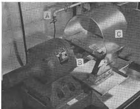
FIG. 11. Trim saw for dicing wafers. Table and wafer are rocked into blade. (A) Coolant system; (B) shallow felt filled reservoir for coolant; (C) coolant shield.
