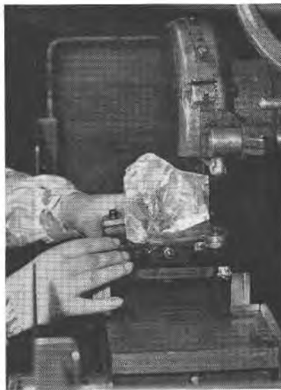
FIG. 4. Milling machine converted for quartz cutting.
