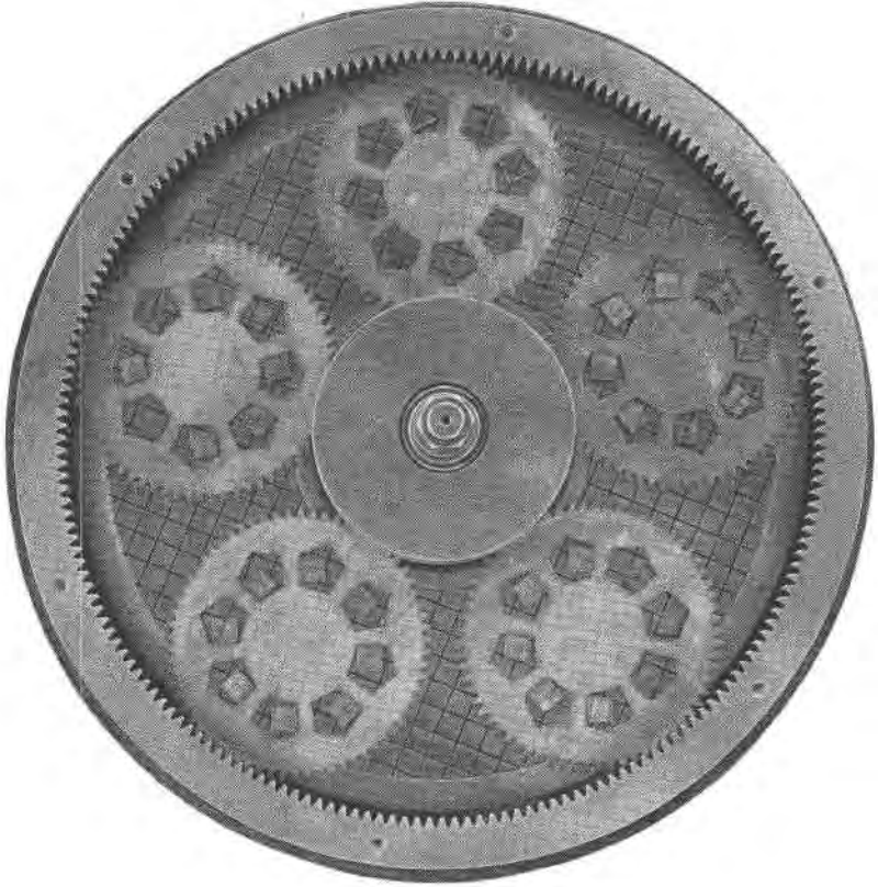
FIG. 3. Top view of planetary lap with upper lap plate removed showing crystals and work-holders.
