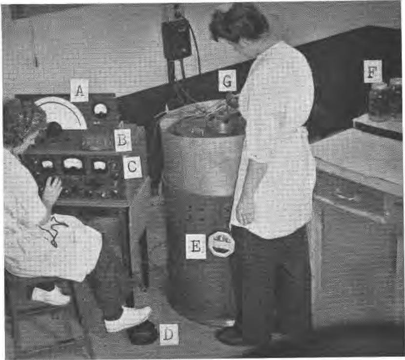
FIG. 4. Planetary lap equipment. (A) Channel sorter, (B) button electrode and anvil, (C) radio receiver, (D) foot switch for lap, (E) variable speed control for lap, (F) abrasive containers, (G) abrasive dispensers.
