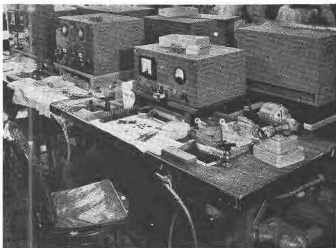
FIG. 8. Final etch finishing position. Note plastic tongs for immersing crystal in Pyrex bowl of etch solution, toothbrush and bowl of soap solution for cleaning, air gun, bowl of dilute ammonia water, comparison oscillator, and abrasive lined cylinder for beveling crystal edges.
