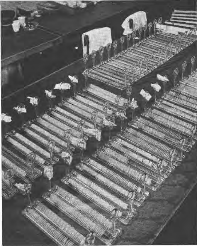
FIG. 7. Crystals racked in notched Pyrex trays, preliminary to being transferred successively to shallow tanks containing sulfuric-chromic acid cleaning solution, running rinse water, etching solution, and running water for final rinsing.
