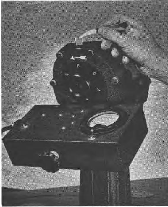
FIG. 14. Close-up view of jig used to hold and oscillate crystals during irradiation.
