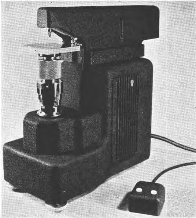
FIG. 1. Tukon testing machine, showing Knoop indenter and rising platform on which specimens are tested.
