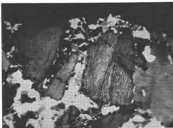
FIG. 3. Fractured huebnerite crystal showing displacement of the several fragments and filling of the fractures by coarse-grained quartz. Laths of sericite replace the quartz filling, and narrow rims of scheelite surround the fragments of huebnerite. Crossed nicols, \times 34 .
