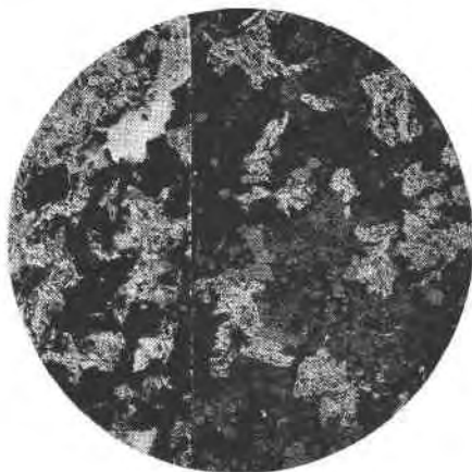
FIG. 1. (Right). Sagenitic rutile in chlorite rock. Light gray, rutile; medium gray, magnetite; black with lustre, chlorite. (Left). Rutile in pocket with apatite. White is apatite. Photo of polished slabs about \frac{2}{3} natural size.
