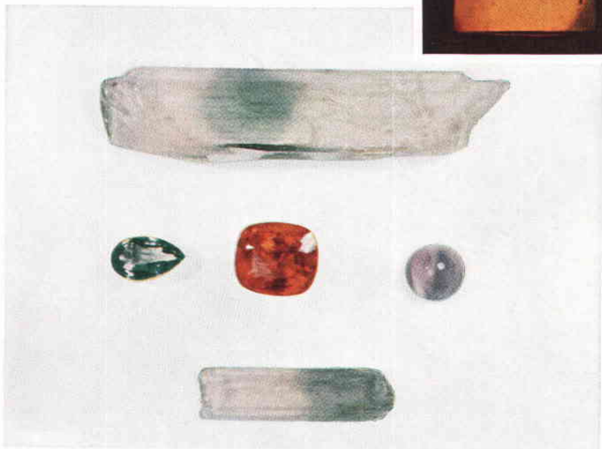
FIG. 3. Specimens of Fig. 1 after treatment, in whole or in part, by five minutes irradiation from new x-ray tube.
