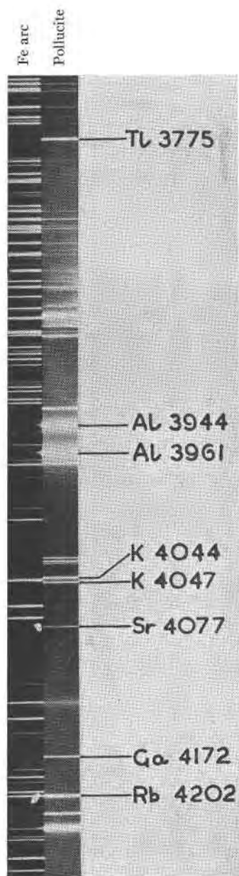
FIG. 1. Spectrum of residue of a specimen of pollucite (Karibib, South West Africa) after treatment with hydrofluoric acid. Note strong relative intensities of Sr 4077 and Al 3944 compared with the weak intensities of these lines in Figure 2. It is probable that the emission of Sr 4077 is from radiogenic strontium (Sr 87 ).
