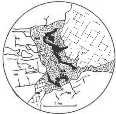
FIG. 2. Drawing of thin section from the 2113 level in the footwall ore zone, showing magnetite (black) in the crushed anhydrite (can) zone as well as a tongue into the anhydrite (an) crystal. Aegirinaugite (ae)
