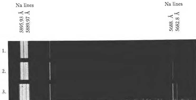
FIG. 1. Spectrograms of (1) schroeckingerite, (2) synthetic mixture of U_3O_8 and CaCO_3 containing 3.6 per cent Na_2O and (3) the synthetic mixture with 7.3 per cent Na_2O .
